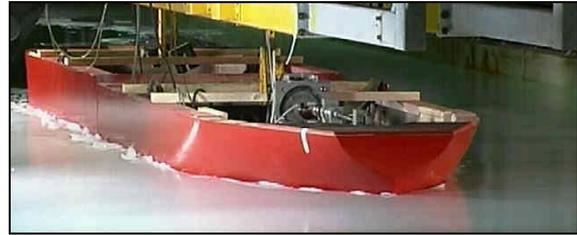
**Figure 20, Model running astern in level ice**
