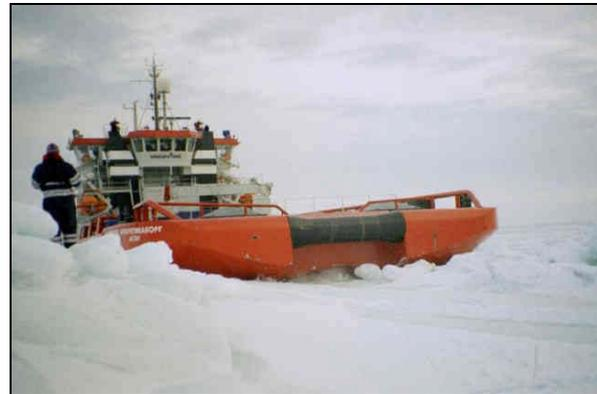
Figure 11, IBSV Antarcticaborg penetrating a 7 m thick ridge running astern.
