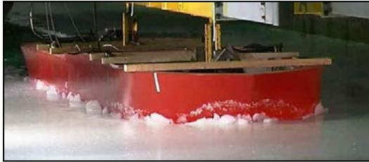
**Figure 19, Model running ahead in level ice**
