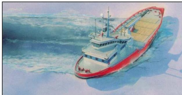
**Figure 27, Oblique icebreaker making a wide channel**
