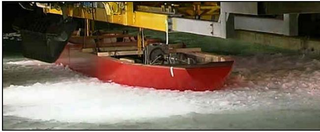
Figure 24, Model in ridged ice
