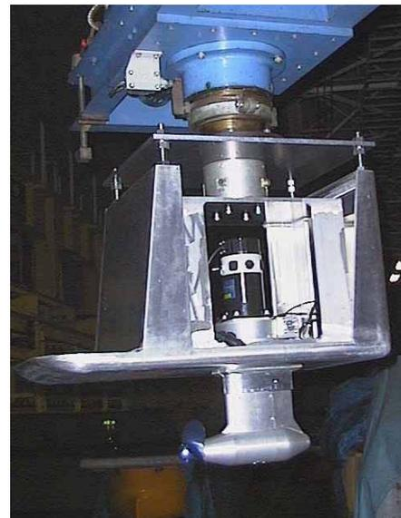
Figure 18, Pressure distribution (Panel Method) and pod open water test unit
